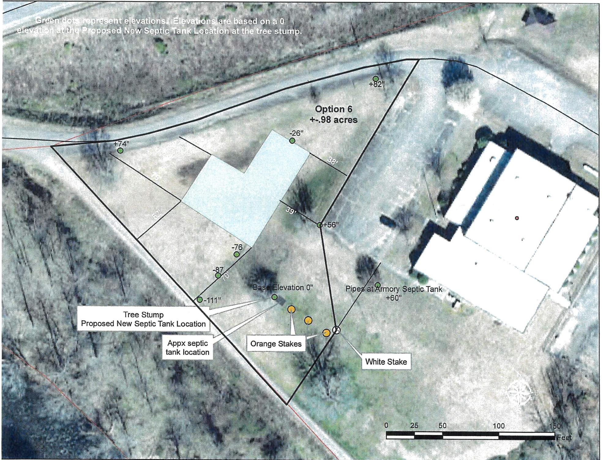
Green dots represent elevations. Elevations are based on a 0 elevation at the Proposed New Septic Tank Location at the tree stump.
